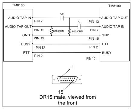
For voice linking applications the value of Cc should be at least  $100\eta F$ .
